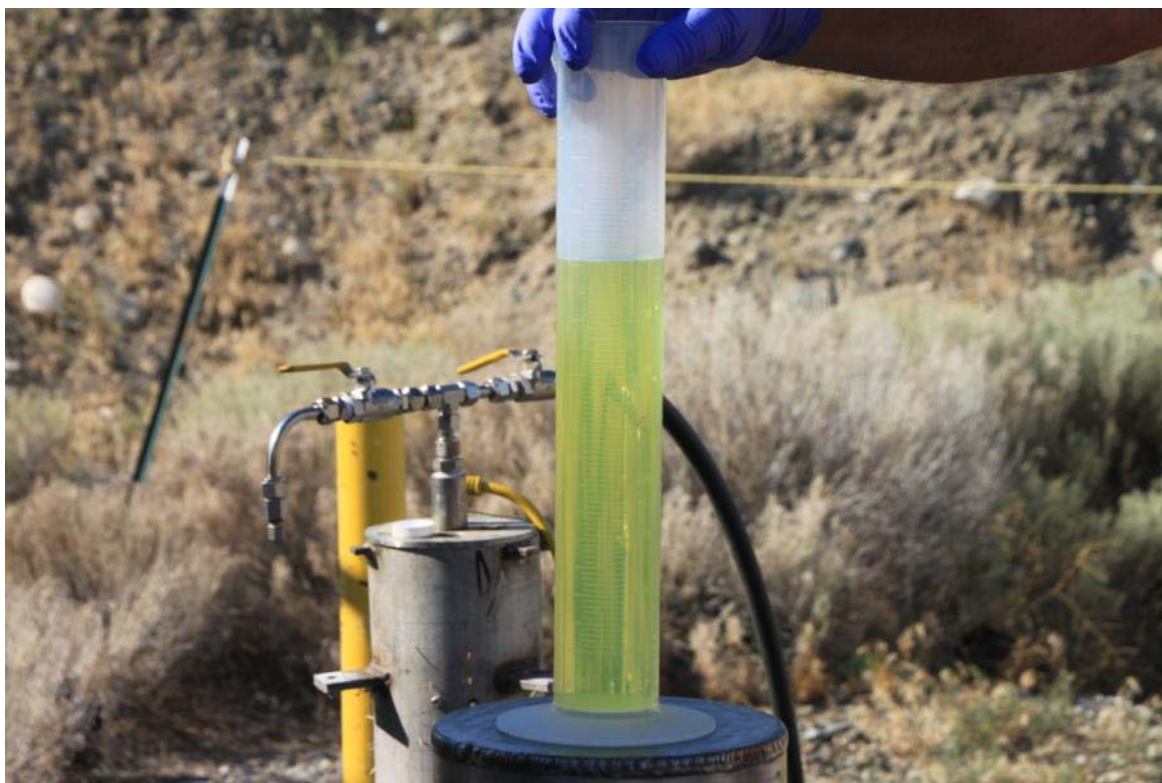
Samples of hexavalent chromium are removed from wells in the 100 Area as part of the groundwater treatment program.
