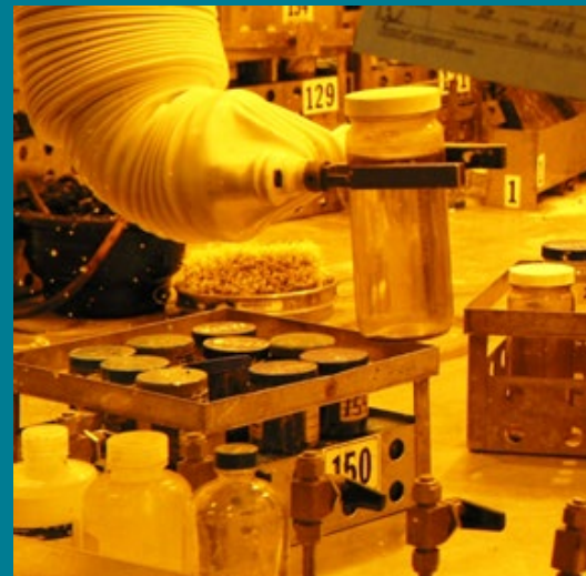
The laboratory has 11 hot cells, which allow crews to remotely handle and analyze radioactive samples.
