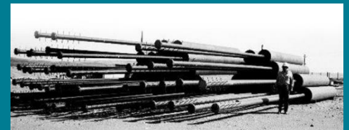
Air lift circulators before installation into waste tanks. Man on right for size reference.
