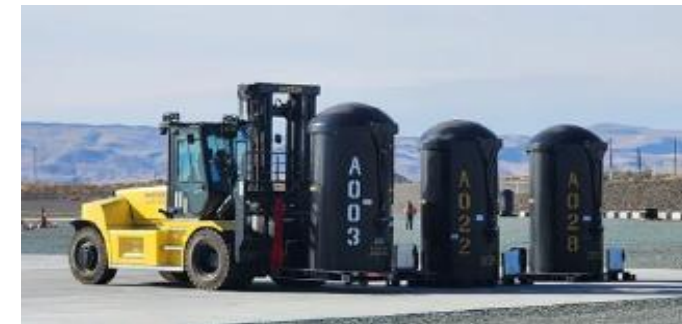
First shipment of immobilized low-activity waste placed on the Integrated Disposal Facility storage pad
