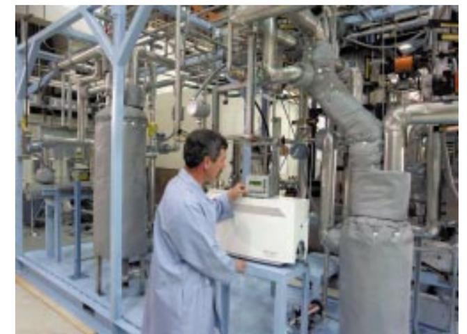
During tests that proved the effectiveness of the spent nuclear fuel drying process, Engineering Technician Mike Dahl checks instrumentation on the first cold vacuum process unit
