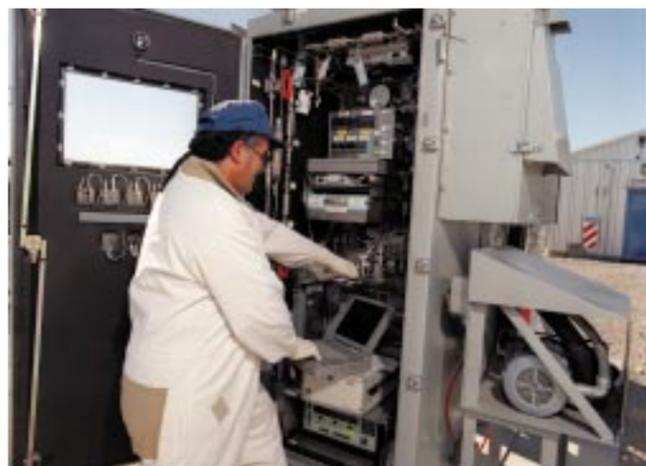
TWRS workers installed hydrogen monitoring systems and other safety devices to gather key data on flammable gas behavior
