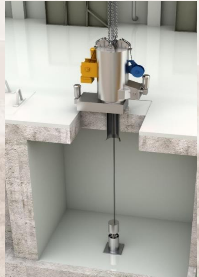
Depiction of transfer system used to lift sleeves out of Hot Cell G
