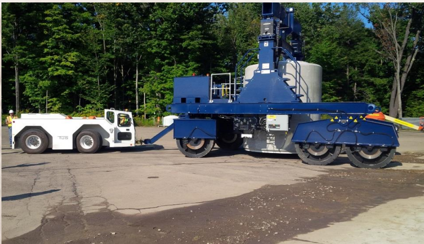
Representation of a vertical cask transporter
