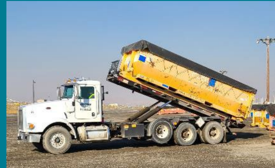
Rolling containers are used to offload bulk waste into the facility's disposal cells.
