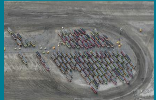
Environmental Restoration Disposal Facility containers are weighed, characterized and staged for disposal.
