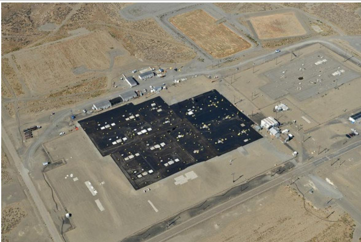
Aerial of previously installed surface barrier at another tank storage area (TX Tank Farm).
