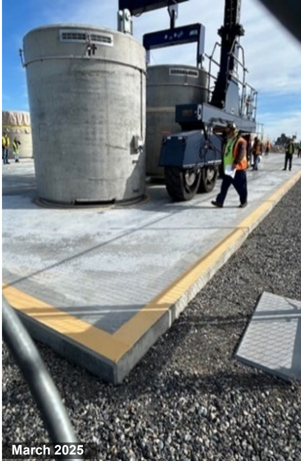
Workers at the Waste Encapsulation and Storage Facility practice moving a cask
