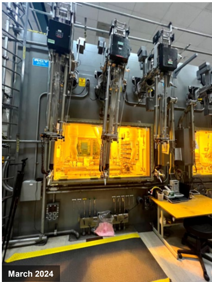
Crews removed old glass windows from Hanford's 222-S Laboratory 11A hot cell and replace them with new windows.
