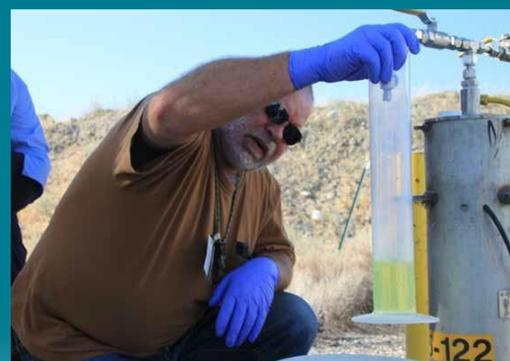
*Groundwater containing the contaminant hexavalent chromium is sampled from wells near the Columbia River.*
