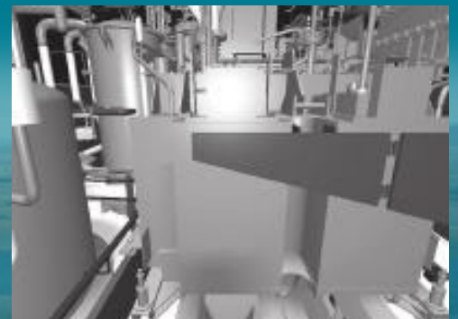
Two 90-ton melters will produce a sturdy glass product in the High-Level Waste Facility.
