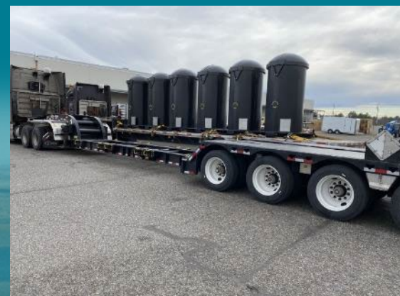
A special waste transporter will carry waste containers to the Integrated Disposal Facility during direct-feed low-activity waste operations.
