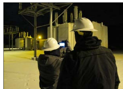
Infrared inspection of electrical transmission system
