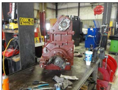
Leaking pump gear box repairs on HFD engine
