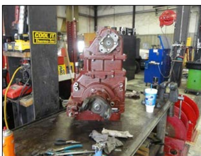
Leaking pump gear box repairs on HFD engine
