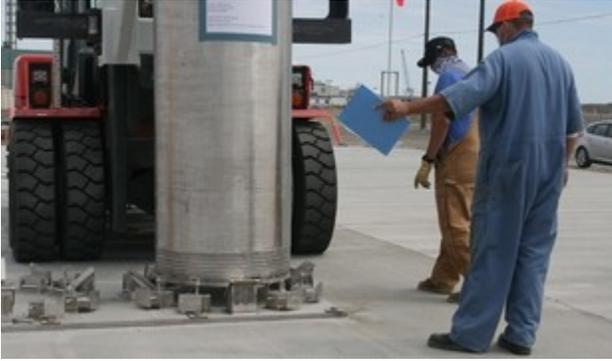
*Crews with Washington River Protection Solutions place a mock-up ion-exchange column onto a storage pad during column replacement testing at the Hanford Site.*
