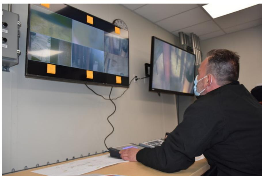
*Dave McCary, a nuclear chemical operator for Department of Energy contractor Washington River Protection Solutions, maneuvers robotic sluicing equipment to remove waste from Tank AX-104, one of four single-shell tanks that make up the AX Tank Farm. Each of the tanks has a capacity of 1 million gallons.*
