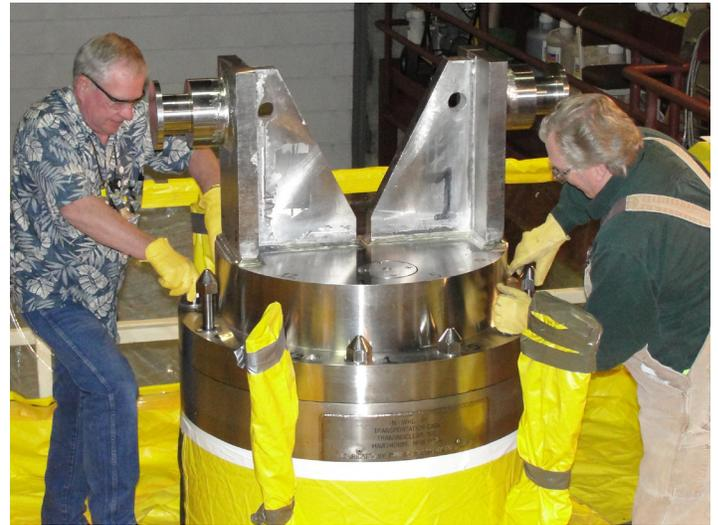
The container was then transferred to the Cold Vacuum Drying Facility adjacent to the K West Reactor where it was purged with helium gas to vacuum dry the fuel. The container was then shipped for interim storage at the Canister Storage Building until a disposal alternative is available.
