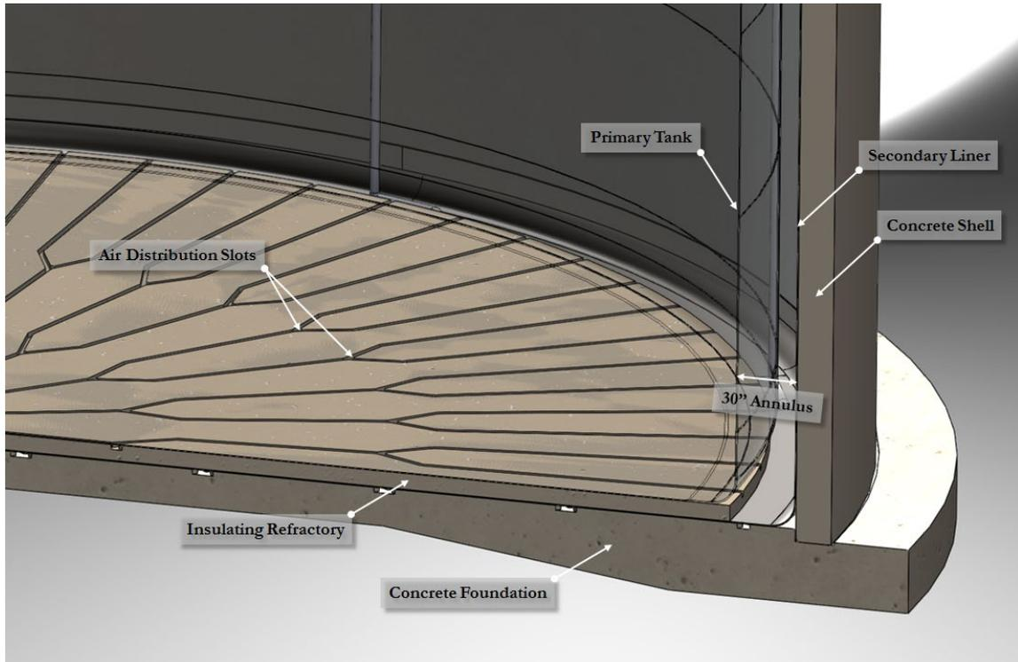
Figure 1. Double-Shell Tank General Features
